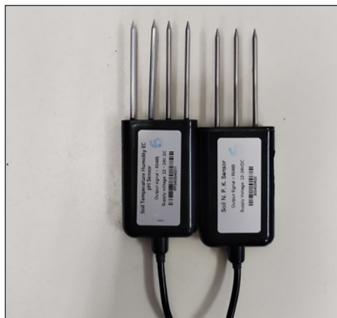
Figure 2. Stainless steel soil NPK, temperature, moisture, EC and pH electrical probes
